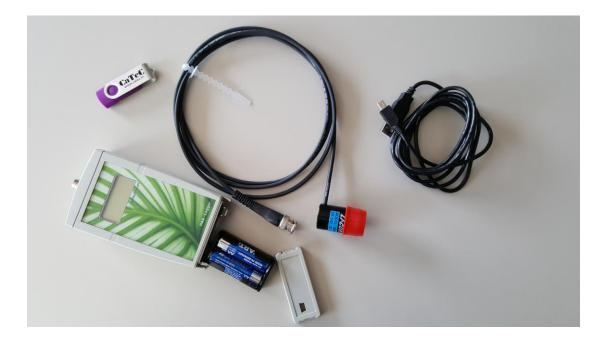
To prevent that the PAR-LOGGER is switched off while logging, the on/off switched is mounted so that the button has to be pressed quite deep to switch the PAR-LOGGER on or off. You can feel it and hear it when the switch toggles. Press the small black button far enough with your nail or a pencil until you feel and hear it switch.
